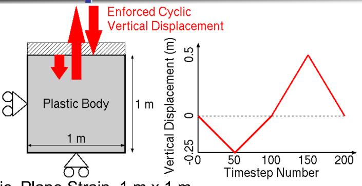
■ Static, Plane Strain, 1 m x 1 m
