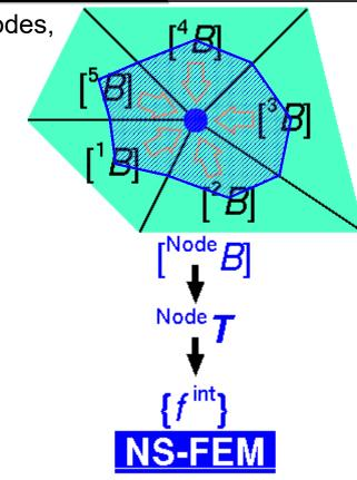
close to FVM with vertex-based control volume
