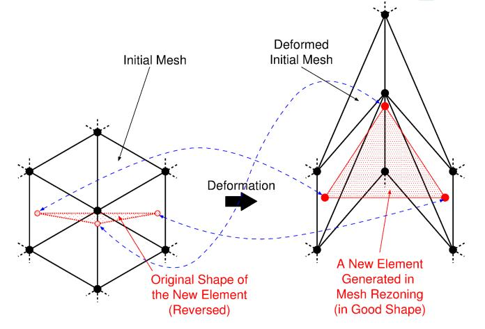
Remeshing on too distorted mesh brings "originally reversed elements".
