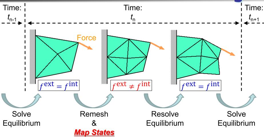
The way of mapping varies with the material constitutive model. (e.g. Elasto-plastic models necessitate some kind of correction.)
